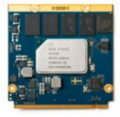
The H6089 is a compact (70mm x 70mm) high-performance, low power COM module based on the Intel® Atom® Elkhart Lake Systemon-Chip. The SOC have the 11<sup>th</sup> generation Intel® UHD Graphics Engine GPU built in along with a dual or quad core CPU and I/O controller.
