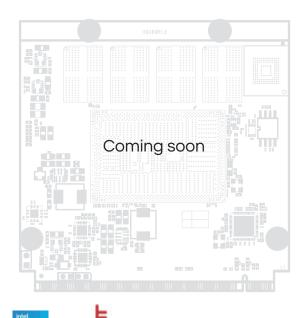
The H6089 is a compact (70mm x 70mm) high-performance, low power COM module based on the Intel® Atom® Elkhart Lake Systemon-Chip. The SOC have the 11<sup>th</sup> generation Intel® UHD Graphics Engine GPU built in along with a dual or quad core CPU and I/O controller.
