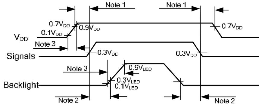
Note 1: In order to avoid any damages,  $V_{DD}$  has to be applied before all other signals. The opposite is true for power off where  $V_{DD}$  has to be remained on until all other signals have been switch off. The recommended time period is 1 second.
