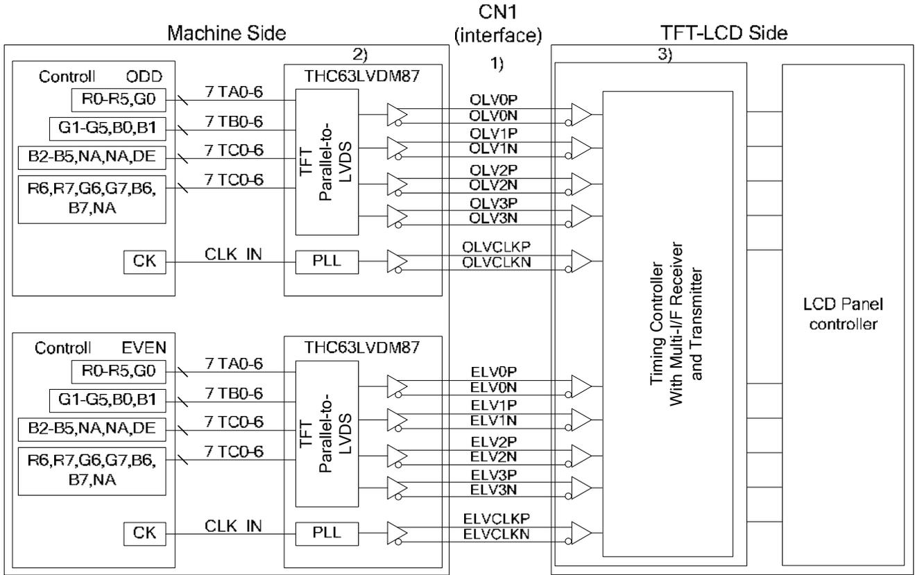
Note 1: LVDS cable impedance should be 100 ohms per signal line when each 2-lines (P, N) is used in differential mode.
