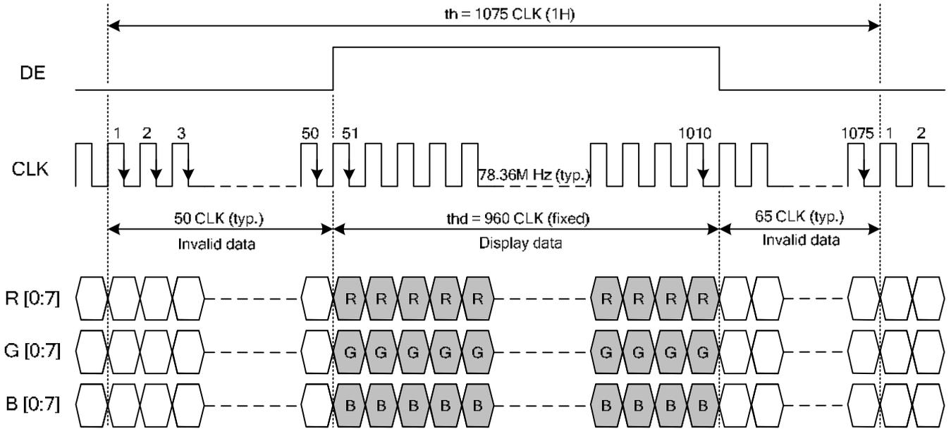
Fig. 9.1 Horizontal Timing
